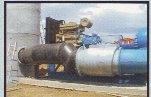
Irrigation pump - NSW cotton fields. 28" ID seal able to withstand 20 foot of head of water.
